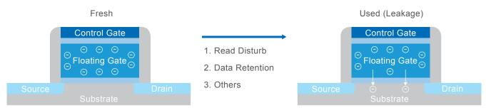
Potential Failure Mechanisms
